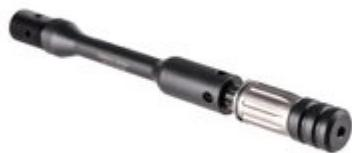
\* Vepr and Saiga Pistons will require drilling through the op-rod after screwing the piston into the carrier, due to variations in the staking location. These Op-Rods are Phosphated instead of Nitrided to allow easy drilling.\*
